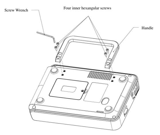
Figure 1-5 Handle Installation
