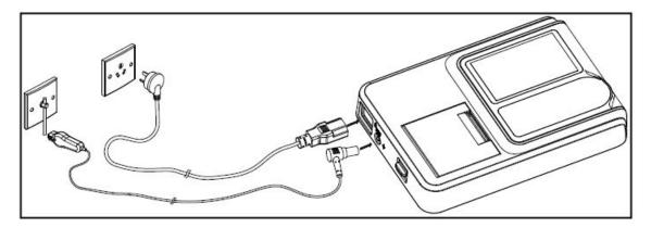
Figure 2- 2 Connect to AC Power Supply
