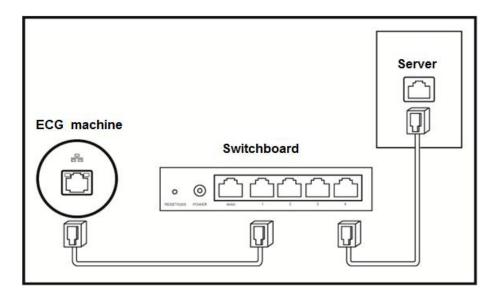
Figure 2- 4 Cable Network Connection
