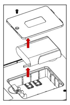
Figure 7- 1 Battery Replacement
