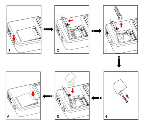
Figure 2- 1 Install the Recording Paper
