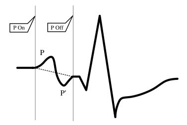
P On is the starting position of P wave, P Off is the ending position of P wave, and dashed line is the reference baseline
