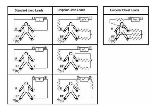
Figure 2- 5 Lead Connection
