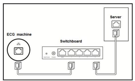
Figure 2- 4 Cable Network Connection
