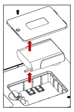
Figure 7-1 Battery Replacement
