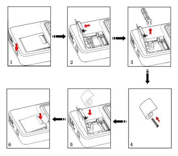
Figure 2-1 Install the Recording Paper
